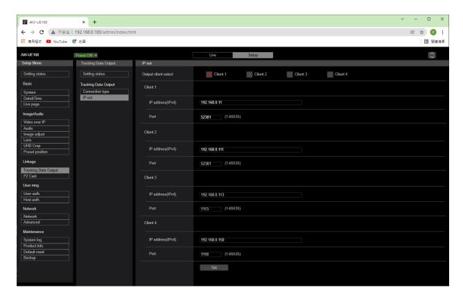
Go to the Setup / Tracking Data Output / Connection Type page and set the IP(UDP) mode
