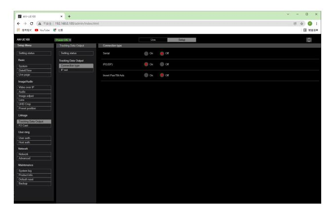
**Second** – You need to setup same framerate on all devices: cameras, capture boards and monitors. Otherwise smooth movements on your video will be impossible to obtain. For Forward boards (FDExt) you need to run FDConfig2 and set the frame rate to the same as the FreeD camera.
